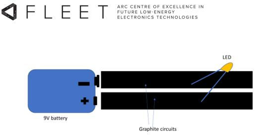
Figure 1. Graphite circuit with a 9V battery and LED
